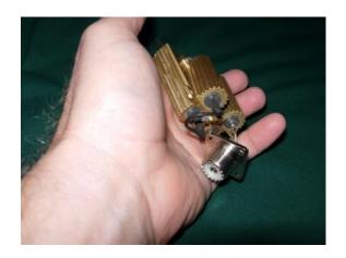
Unfortunately it also has about 80 microhenries (80µH) worth of inductance. So it's pretty obvious that a non-inductive resistor is needed. Capacitance can also cause reactance and non-linear impedance in a load but nowhere near the extent of inductance.
