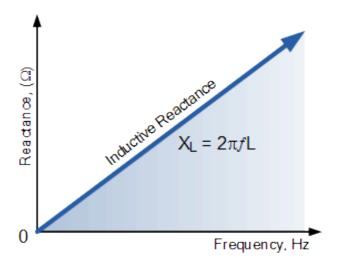
Most common power resistors are wire-wound, which have significant inductance. So RF dummy loads must use resistors with little or no inductance.
