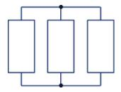
From this simple schematic we intuitively see that the voltage across parallel components must be the same.
