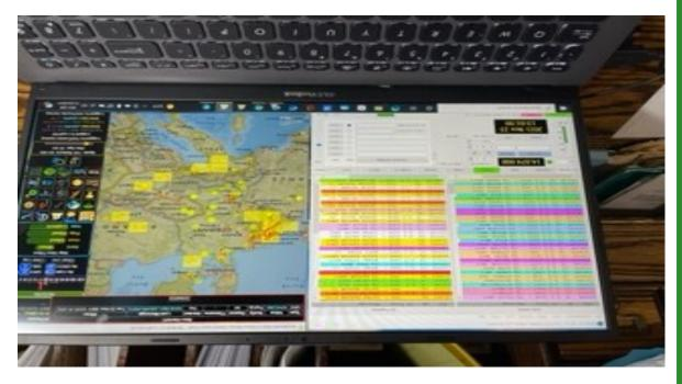
After a lot of trial, error and perseverance I finally got FT8 up and running. I installed Grid Tracker and Dimension 4 (for time synchronization) along with it. FT8 is designed to maximize communication even when signals are very weak (as low as -24db). This means that even low powered stations and stations with sub-optimal antennas can make contacts worldwide. You can choose to either call CQ or choose and pounce.
