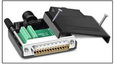
which pin a colored wire in a preexisting cable connects to. No worries about insulating those tiny, soldered wires from each other. You can use larger wires so no more breaking off the meager five or six strands of thin copper inside individual data lines while stripping them of insulation. And if you wire incorrectly, you can easily switch a wires pinout. Just strip a wire end, push it into the numbered connecting point, and tighten the screw. Wrong pinout?
