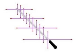
Extending our VHF or UHF range can be achieved without infrastructure, by using yagi antennas. Although this type of antenna can help radically increase the range of VHF and UHF signals, it also adds to the amount of equipment we carry.
