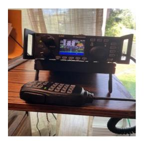
I recently added a Xiegu G90 to my shack. It is an small portable HF radios that has a onboard tuner (that works great), waterfall. CW decoder, two VFO's, memory presets, detachable head, very good on power usage (I have been operating it on my 20 amp LifePo4 battery for two hours a day for several days and used less than .2 amp.) Look if up on eHam.com. It's a great radio for its price point, \$440.00.
